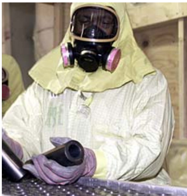
A HazWat inventories and repackages depleted uranium cores. Photo Courtesy of Fernald Photography
