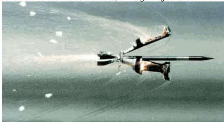
Armor Piercing Fin Stabilized Discarding Sabot rounds (aka. sabot rounds) with DU penetrators Photo courtesy of Department of Defense
